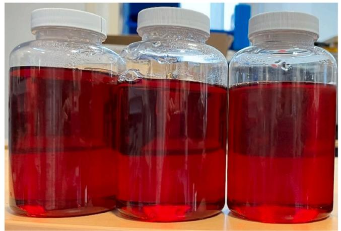
Fig. 1. TruView gel from the same batch packaged in three 400 ml cylindrical jars partially filled.
