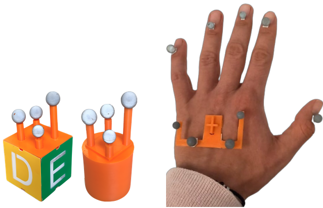
Fig. 3: On the left, the markers are placed on two different objects, while on the right, the markers are placed on a hand. The back of the hand and the two objects have multiple markers on rigid supports for tracking their orientation.
