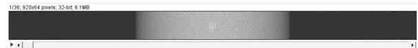
Figure 3: Projection of a water cylinder of 10 cm diameter with a central copper cube
