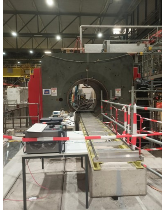
Figure 4: CB100 experimental run March 2023 inside Morpurgo magnet with 1.6 T magnetic field over 21 days at CERN
