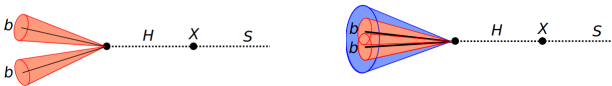
Figure 2: Sketch illustrating the collimated b -jets resulting in their reconstruction in a single jet when m_S \ll m_X (right) as opposed to the separated b -jets (left).
