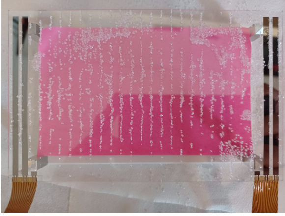
Figure 6: Haptic system covered with sugar and activated at the frequency corresponding to the focused Lamb's mode. The sugar concentrates at the vibratory nodes, creating a Chladni pattern.
