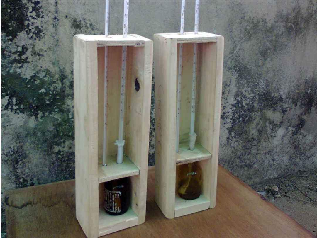
Figure 5. Locally constructed Hygrometer
