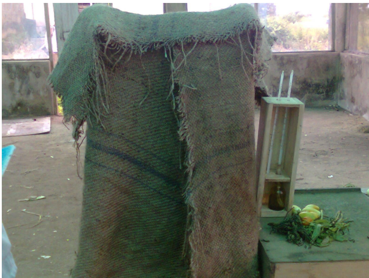
Figure 6. Locally Constructed Evaporative Cooler For Agric Produce Storage
