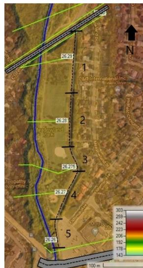
**FIGURE 2.** Etobicoke Creek levee segments numbered 1 to 5 ; in blue Etobicoke Creek flowing southward ; in green the hydraulic model cross-sections
