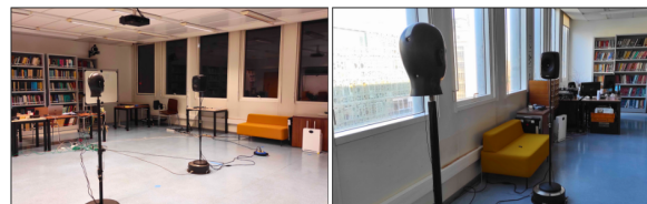
Fig. 1: Measurement setup in \mathbf{Pos}_{center} (L) and \mathbf{Pos}_{wall} (R) of the test room.
