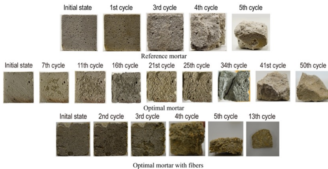
FIGURE 6. Effect of \text{Na}_2\text{SO}_4 solution on the aspect of the different mortars after curing time of 1 month.
