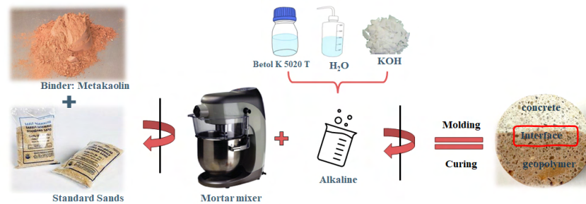
FIGURE 1. Geopolymer Mortar Preparation Flowchart
