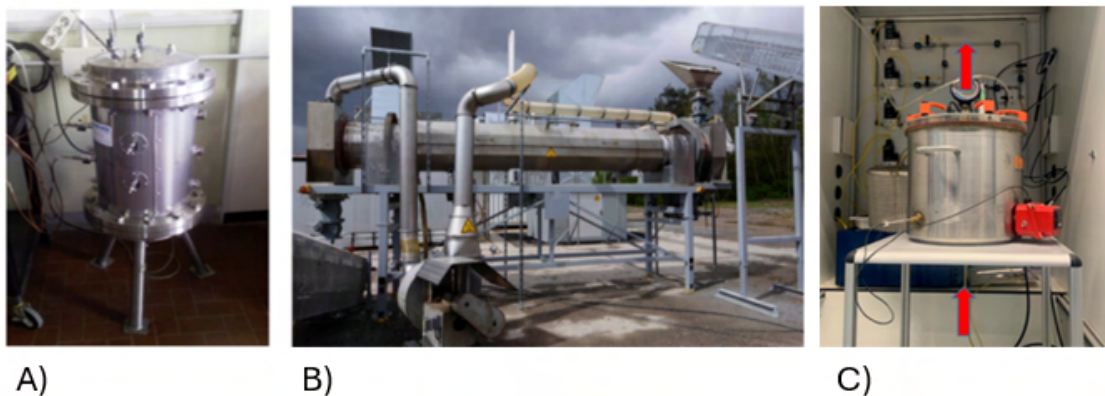
Figure 2 : (A) laboratory-scale reactor (Lombardi et al., 2016) ; (B) industrial scale reactor (Schnabel et al., 2021) (C) Carbonation reactor in our laboratory at ESTP.
