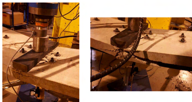
FIGURE 5. Crushing of the concrete central block due to cylinder punching, phase (c)
