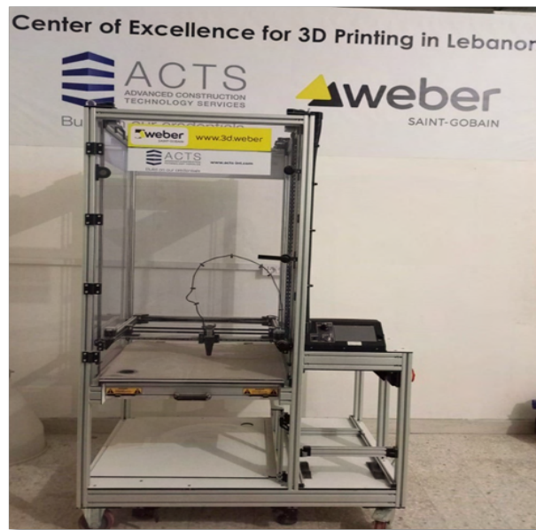
Figure 5. The gantry-type printer used in the current study
