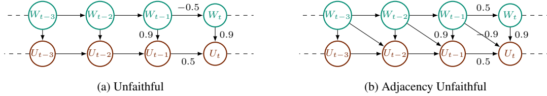
Figure 2: Illustration of the violation of the faithfulness and the adjacency faithfulness assumption. (a) violates the faithfulness assumption but satisfies the adjacency faithfulness assumption and (b) violates the adjacency faithfulness which implies that it violates the faithfulness assumption.
