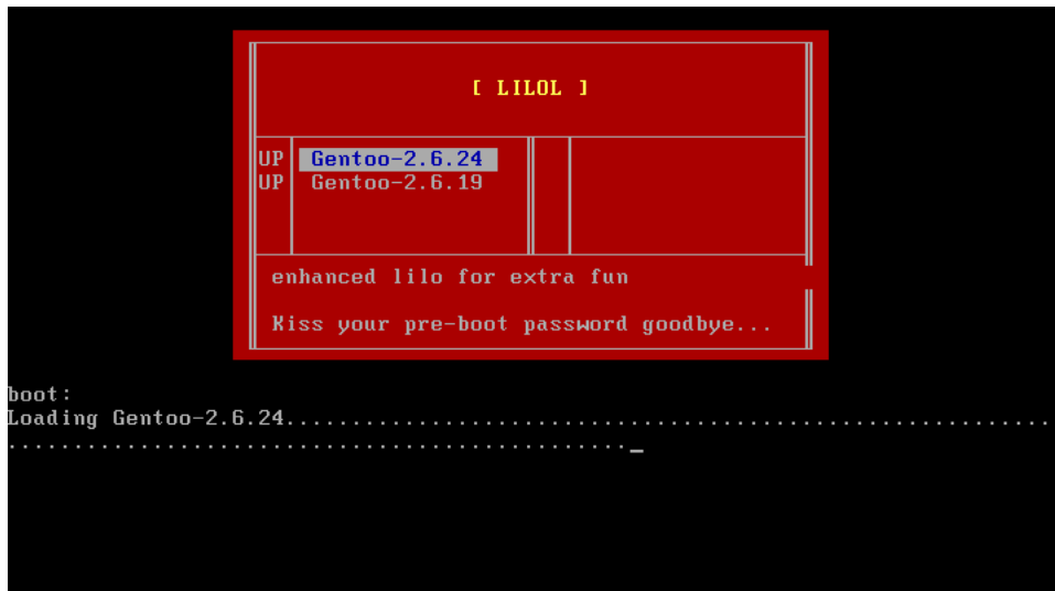
Fig. 15. Patched lilo rebooting without prompting for a password.
