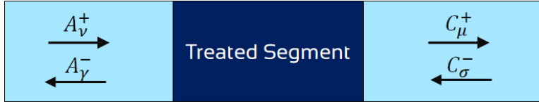
Figure 1: Illustration of the scattering problem in acoustic waveguide, with guided modes amplitudes definition on the left side, and on the right side of the acoustically treated segment.
