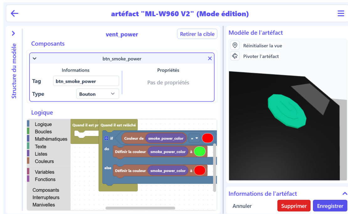
Figure 3: Screenshot of HELP XR interface for the artefact configuration and visualization
