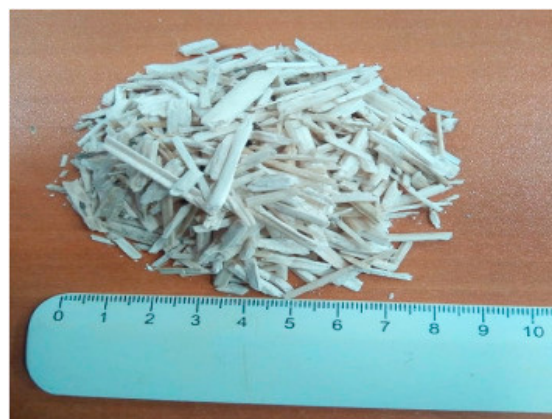
Figure 5. Hemp shives in bulk with a diameter of 1 cm [50].
