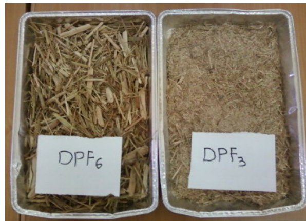
Figure 8. Date palm fiber with two different dimensions, DPF 3 (3 mm) and DPF 6 (6 mm) [77].
