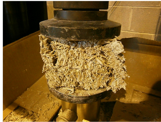
Figure 22. Typical failure of hemp–lime concrete under an axial compressive load [92].
