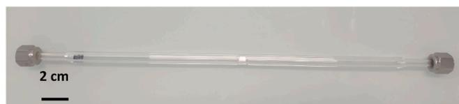
Fig. 8. H<sup>+</sup>-ZSM-5 monolith(A) inserted in a glass tube for the alkylation of toluene by methanol at 350 °C.
