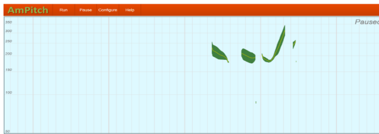
Figure 2: A real-time display of pitch and amplitude in AmPitch of the utterance: “He said what?”
