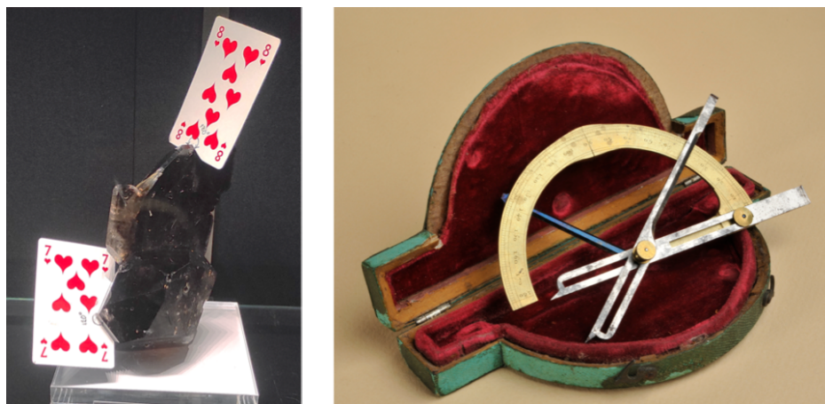
Figure 11. Left: 120° angles in quartz crystals. Right: Carangeot goniometer (C. Basoche property), end of the XVIIIth century, beginning of the XIXth century. © Collection de Minéraux, Sorbonne Université, Paris, France.
