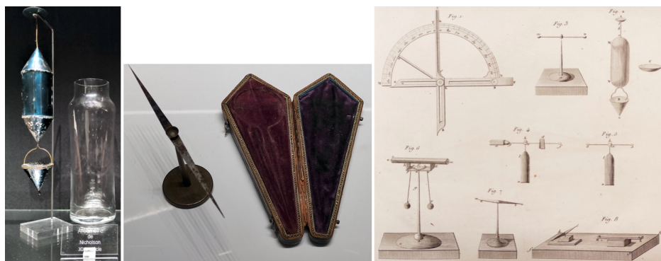
Figure 17. Left: Nicholson hydrometer, XIXth century. Middle: mineralogy compass, beginning of the XIXth century. Right: engraving from the Traité Élémentaire de Physique by Haüy. © Collection de Minéraux, Sorbonne Université, Paris, France.
