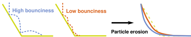
Fig. 4: The coefficient of restitution affects the amount of energy absorbed from the particle when hitting the ground. Here, rain is applied on an initial slope (yellow). Only two particles are displayed, with a high (blue) and low (red) coefficient of restitution. The resulting slope after erosion is displayed in blue and red (right).
