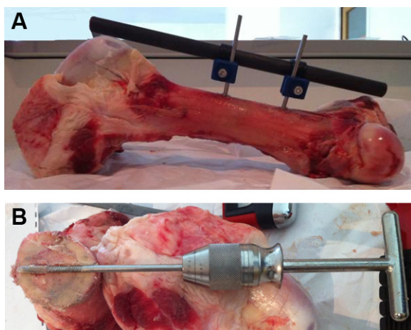
Figure 5 Illustrations of the mechanical test performed. Notes: (A) Image of a unilateral fixator assembly performed on a cow femur. (B) Visualization of the insertion of the pin into the bone on a horizontal section.
