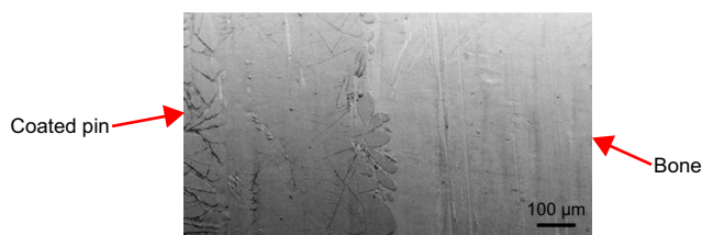
Figure 7 Field emission scanning electron micrograph of the contact area between bone and the coated pin after explantation.
