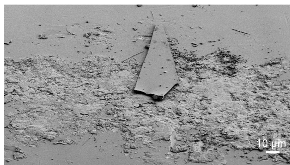
Figure 6 Field emission scanning electron micrograph of the contact area between the grip and the coated pin.
