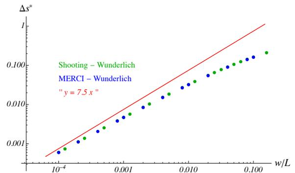
Fig. 10. Size  $\Delta s^*$  of the singular region, where the orientation of the rulings quickly varies (i.e. the inner layer in the Matched Asymptotic Expansion (MAE) calculations). The red line,  $y = 7.5x$ , approximately fits the asymptote of the Wunderlich curve as  $w \rightarrow 0$ .
