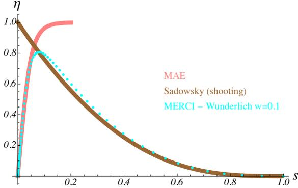
Fig. 29. (blue) Plot of  $\eta(s)$  from MERC1 for the buckled LTB solution with Wunderlich model and constraint  $\eta(0) = 0$ , with  $\Gamma = 30$  and  $w = 0.1$ . (pink) The boundary layer solution from [Audoly and van der Heijden 2022], and (brown) the Sadowsky solution.
