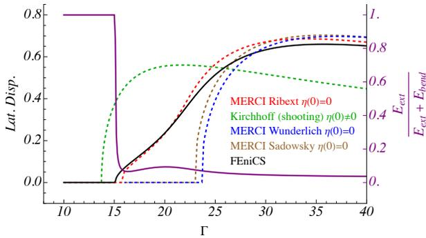
Fig. 22. Lateral Torsional Buckling bifurcation curve with  $\nu = 0.35$ ,  $\frac{w}{L} = 0.1$ , and  $\frac{h}{L} = 0.001$ . Note that in the MERCI-SADOWSKY and MERCI-WUNDERLICH codes, the constraints  $\eta(0) = 0$  and  $|w\eta'(s)| \leq 2$  have been applied. We also plot in purple the ratio of extension energy computed with the FENICS-SHELL code.
