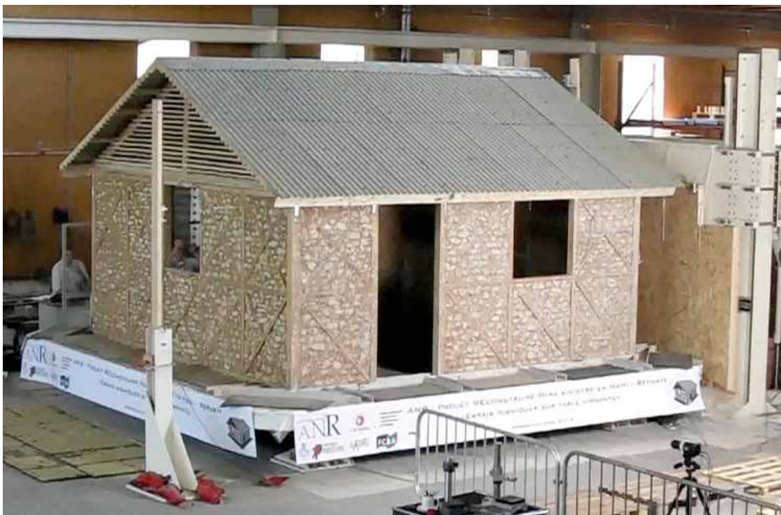
Figure 9: Full scale traditional Haitian timber-frame house with earth and stones infilling tested at FCBA Bordeaux
