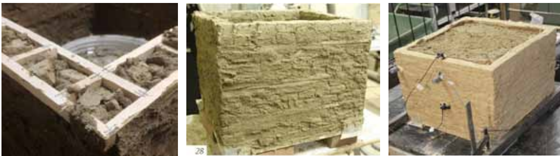
Figure 11: Adobe masonry box model: construction and shaking test
