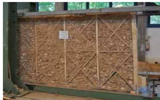
Figure 4: Push over test on a infilled timber-frame shear wall
