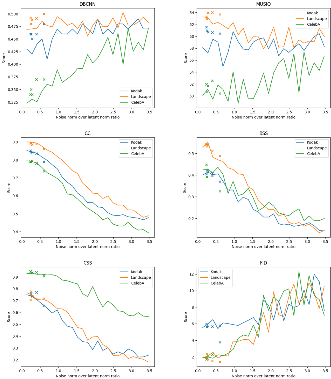
FIGURE 10. Quality and semantic coherence scores, regarding the proportion of noise added regarding the norm of the input latent vector, applied to Landscape, Kodak, and CelebA. Scattered crosses represent the quantized images generated in Section VI-B. (Top to bottom, left to right) DBCNN, MUSIQ, CC, BSS, CSS, FID.
