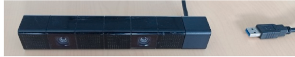
Fig. 5. The used stereo camera is a Sony PlayStation 4 camera model 1. The camera provides two 1280x800 images. The cable was modified to be used on a standard USB3 port.
