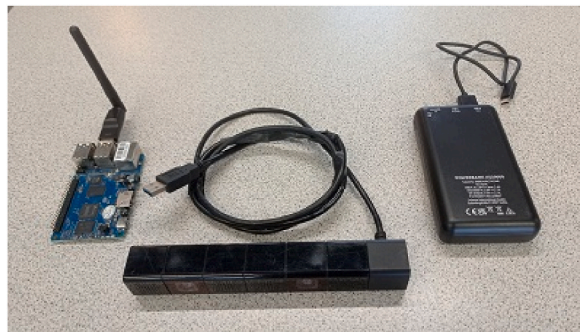
Fig. 19. The complete embedded system. From left to right: a Banana Pi M5 single-board computer equipped with a WIFI dongle and antenna, the stereo camera, and a 20A.h powerbank.
