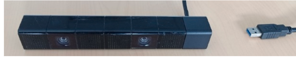
Fig. 5. The used stereo camera is a Sony PlayStation 4 camera model 1. The camera provides two 1280x800 images. The cable was modified to be used on a standard USB3 port.
