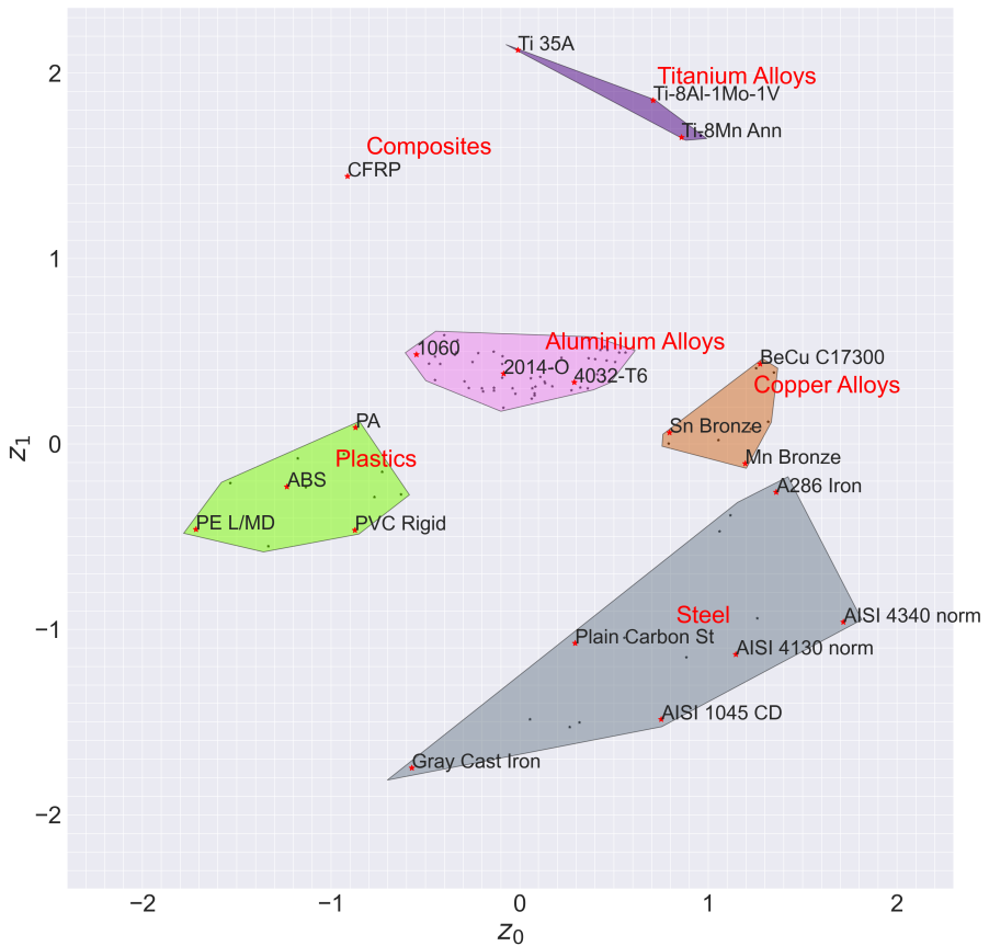
Fig. 2: Material representation in a two-dimensional latent space (7 properties considered)
