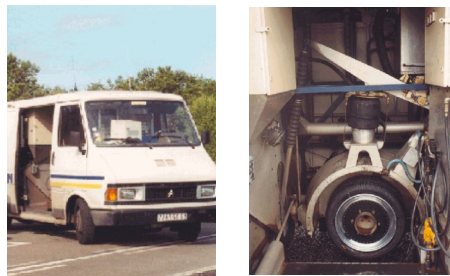
Figure 2. Continuous grip measurement vehicle (CGM); source: [3]
