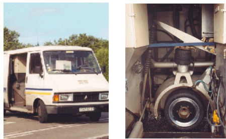
Figure 2. Continuous grip measurement vehicle (CGM); source: [3]
