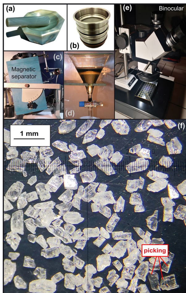
Figure 3. Extraction of fresh feldspars through different steps: (a) crushing, (b) sieving, (c) magnetic separation, (d) sorting by heavy liquid, (e) binocular observation, (f) picking of translucent crystals. All photos taken by Anthony Hildenbrand.
