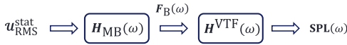
Figure 17. Flowchart depicting the points where the structure-borne quantities are coupled with the respective transfer functions
