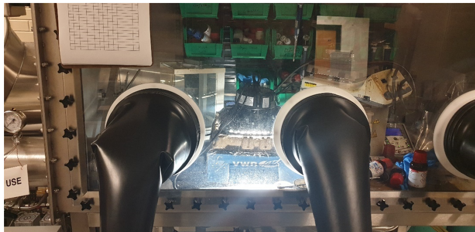
Figure S11: Light illumination of the related thin films was performed under 5000k white LED source (EverWatt, EW-HB-06-V-150W) with 100\text{mW}/\text{cm}^2 intensity in a nitrogen-filled glovebox. The samples were then taken out of the glovebox for measurement after 1-3-6-24 hours of illumination.
