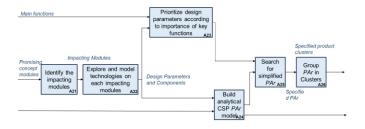
Figure 2: Product Architecture (PAr) generation process
