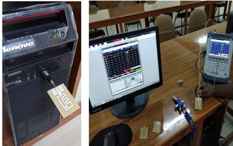
Figure 14. Measurement set up of proposed meander antenna with \lambda/5 dipole
