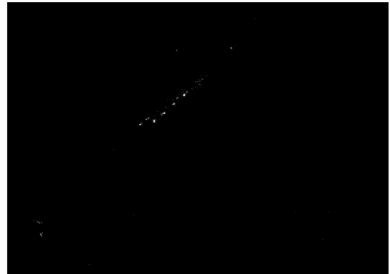
Figure 2. Flashes location map acquired by the GLM sensor at the same date than in Fig. 1. White pixels identify the presence of flashes, and the background is represented with black pixels.
