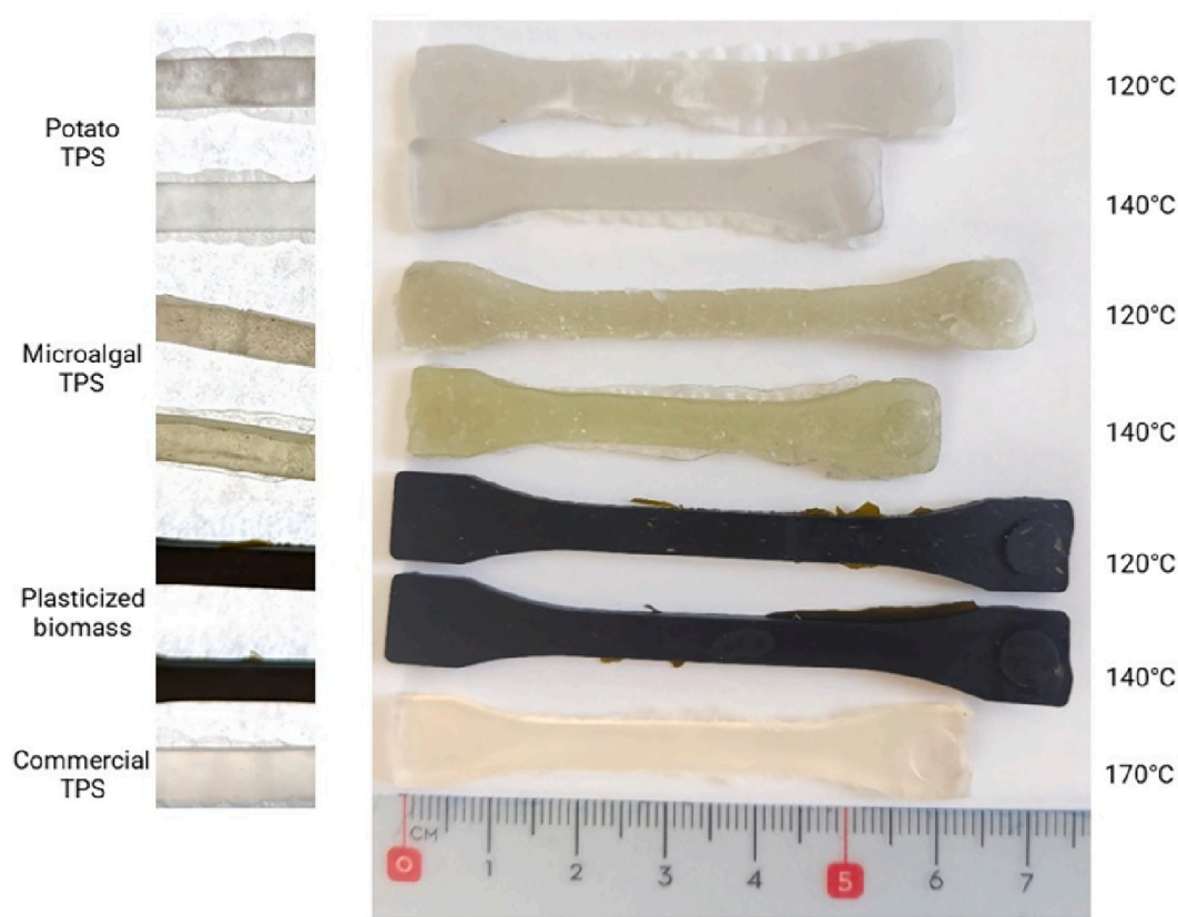
Fig. 7. Injected dogbone specimens of potato TPS, microalgal TPS, plasticized raw biomass, and commercial TPS. On the left picture, dogbone specimens were illuminated from below to expose their transparency and imperfections. The right picture illustrates the length difference between dogbone specimens coming from the same mold. The dogbone mold was 7.5 cm in length, but TPS specimens showed immediate shrinkage after unmolding. The temperatures displayed on the right are extrusion temperatures, all injections being performed at the same temperature of 140 °C.
