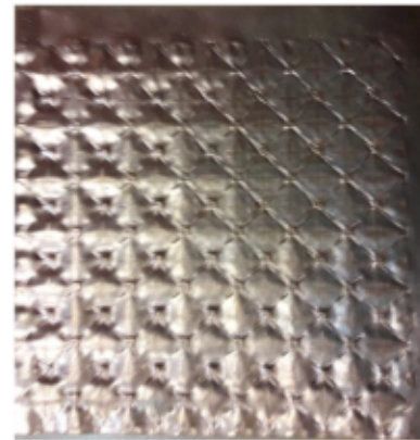
Fig. 5. Workpiece after two passes of the RCS.
