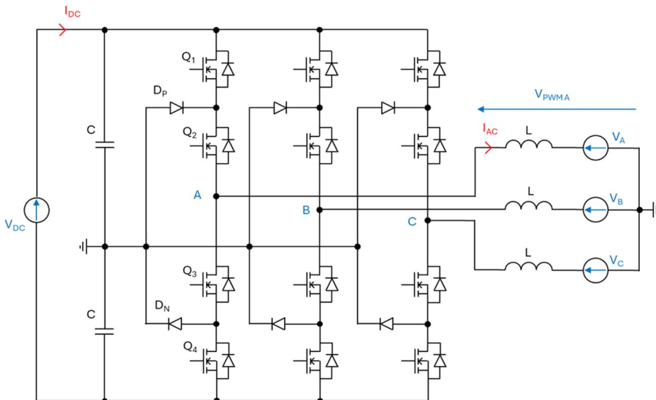
Figure 2 : Structure Neutral Point Clamped 3 niveaux "NPC"
