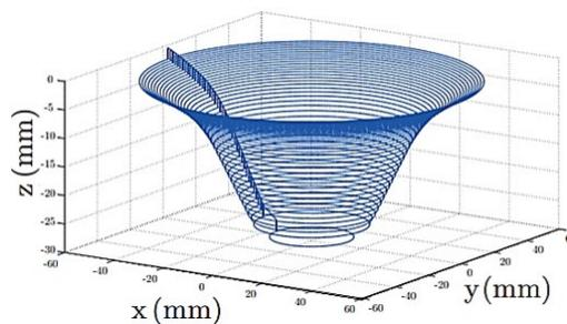
Figure 7: Tool trajectory with successive circular contours
