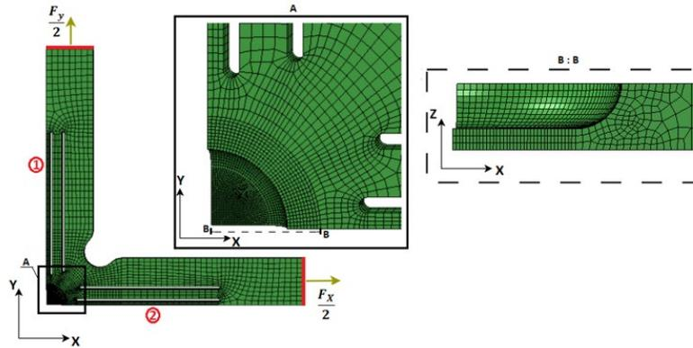
Figure 4: FE model of the cruciform specimen
