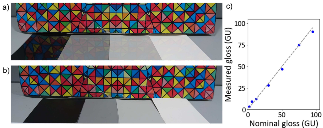
Figure 1. NCS gloss scale samples: optical photographs of (a) full gloss and (b) full mat NCS samples, 2 GU and 95 GU gloss respectively, taken in the photo booth with D65 illumination; (c) measured vs nominal gloss. In (a,b) samples are black, dark gray, clear gray and white from left to right correspondingly.
