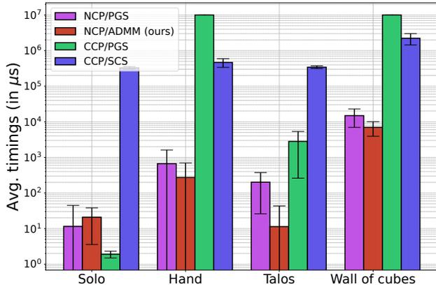
Fig. 5. **Timings on robotics systems.** Thanks to its combination of automatic spectral adaptation (Sec.III-F) and sparse Cholesky update (Sec. III-E), our algorithm (in red) yields a stable behavior across the various robot simulations.
