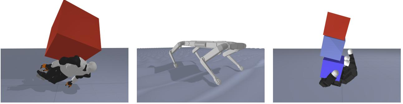
Fig. 3. **Robotics systems.** We evaluate our approach on common robotics scenarios occurring during locomotion, e.g., Talos falling on the ground (**left**), Solo walking on steep terrain (**center**), and manipulation, e.g., Allegro hand interacting with cubes (**right**).
