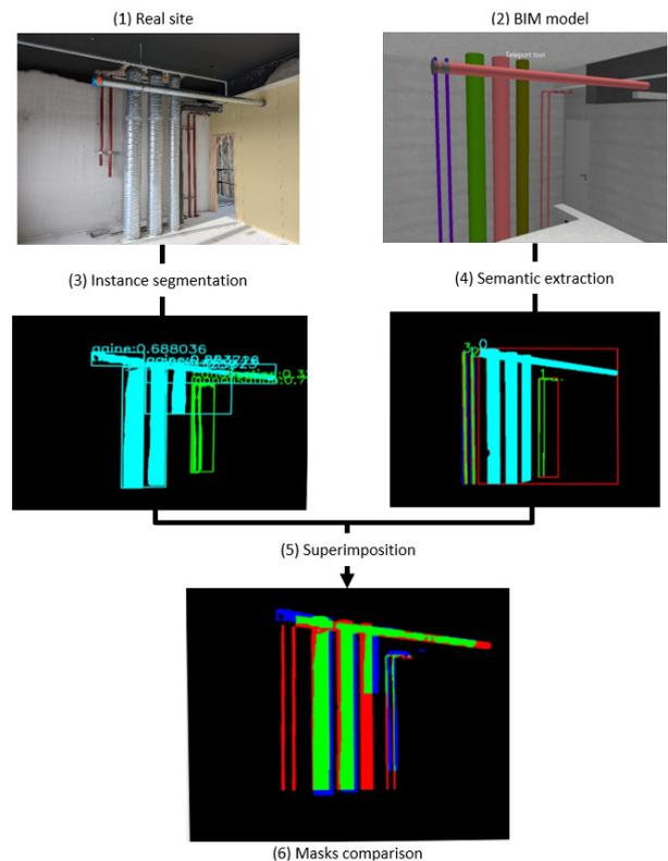
Figure 4. Captured versus BIM comparison.
