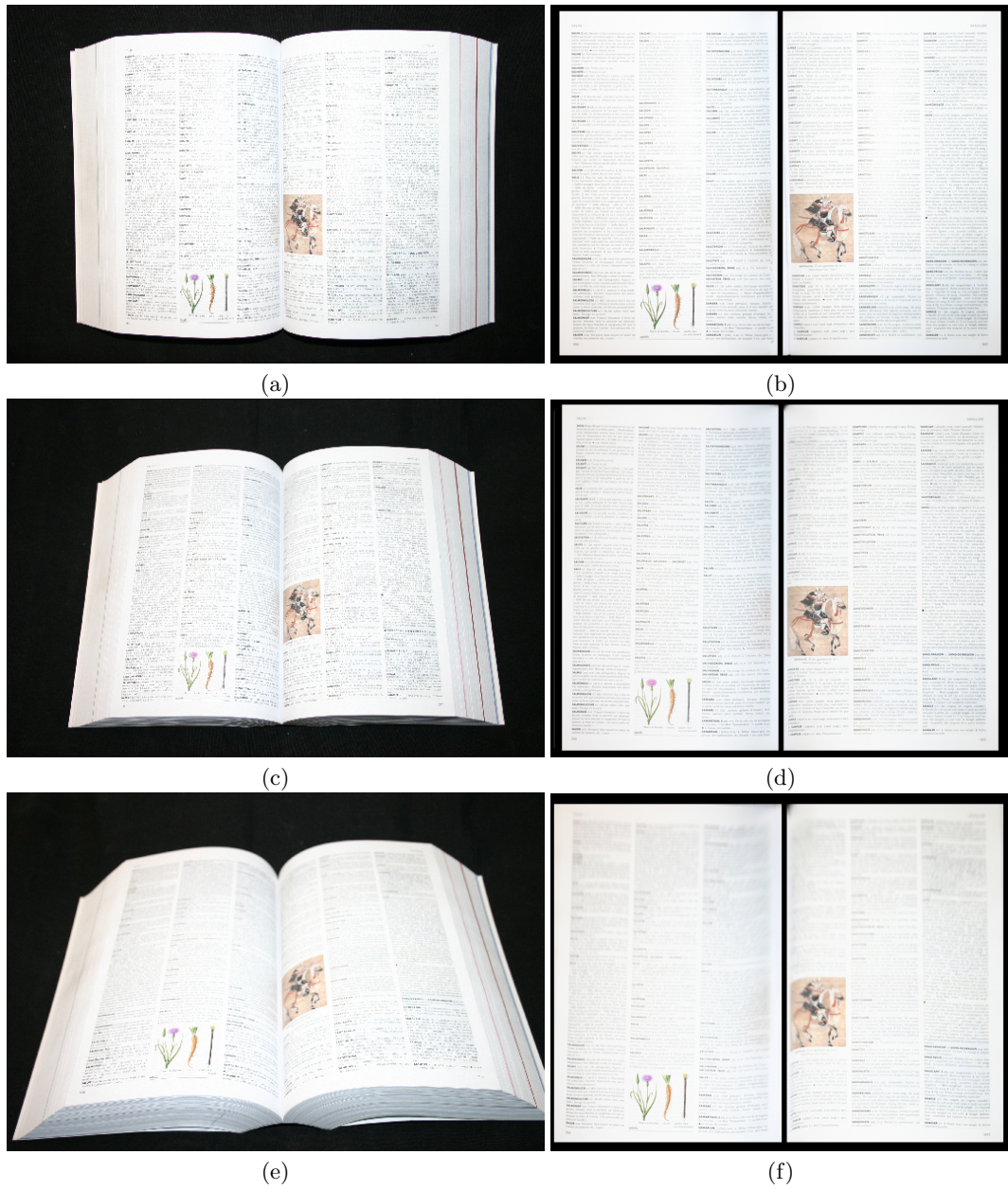
Fig. 3. Three photographs of the same book taken from three different angles of view, and the flattening simulations obtained from each of them: (a-b) \alpha = 1.5^\circ ; (c-d) \alpha = 20.38^\circ ; (e-f) \alpha = 40.54^\circ .
