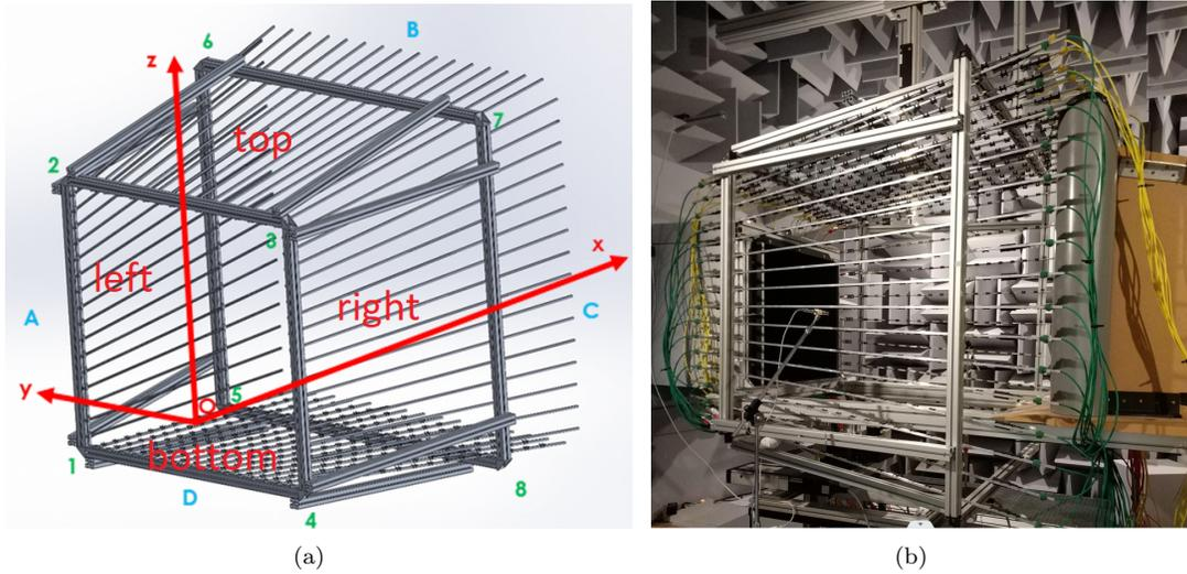
Figure 4: (a) 3D model of the array structure [31]; (b) photograph showing the wind-tunnel components with the installed microphone array. From left to the right are respectively the nozzle, the microphone array and the collector.
