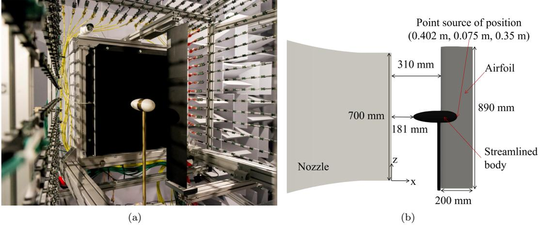
Figure 2: (a) The streamlined acoustic source besides a NACA 0012 airfoil with a finite span in the open test section of the wind-tunnel; (b) sketch of the streamlined body, airfoil and the nozzle of the wind tunnel.
