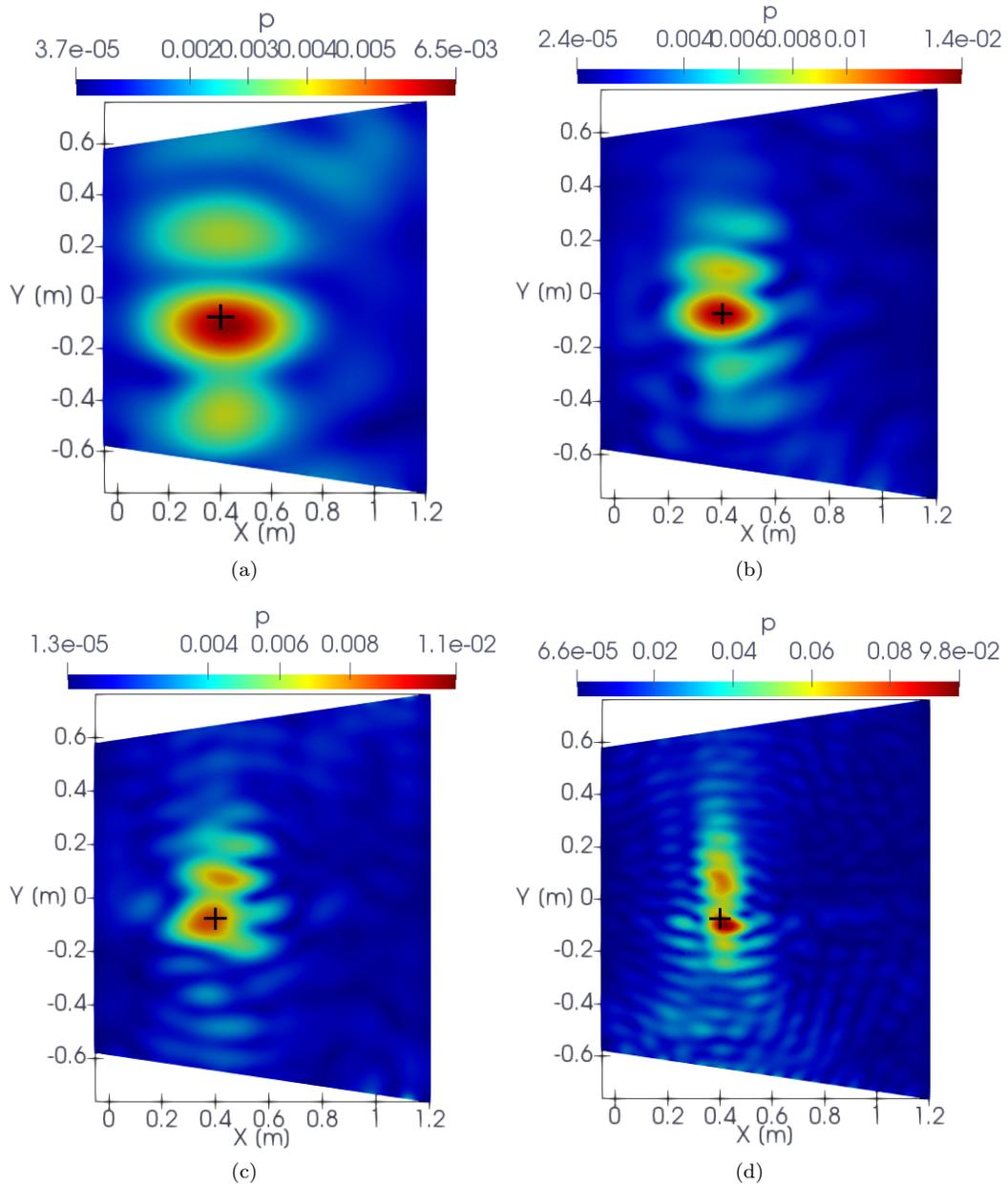
Figure 10: Results of the 3D TR for the synthetic noise source emitted by the streamlined body shown in a planar cross section  $XY$  at  $z = 0.35$  m. 768 channels of acoustic data are used. The solid boundaries of the objects are not considered during the numerical simulation. RMS of the pressure field from 0.005 s to 0.015 s in the third-octave band (a) [561; 707] Hz; (b) [1122; 1414] Hz; (c) [1414; 1782] Hz; (d) [2245; 2828] Hz.
