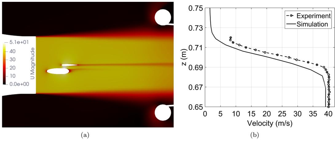
Figure 17: (a) The mean flow velocity of the wind-tunnel flow in a planar cross section  $XY$  at  $z = 0.35$  m; (b) comparison between the numerical result and experimental result for a velocity profile along the  $z$ -direction for a shear layer.
