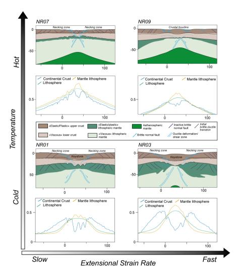
**Figure 7.** Synthetic diagrams showing the various modes of lithospheric thinning and thinning factors during the early development of necking zones depending on the initial Moho temperature and extensional rates.
