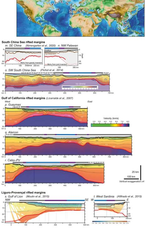
**Figure 1 (cont.).** Crustal scale profiles across rift basins and conjugate rifted margins as imaged by refraction seismic data or modelled from gravity anomalies. This compilation shows the variable geometry of passive margin crustal structure and crustal domains. References are indicated above each profile, their location is indicated on the bathymetric map (after NOAA National Geophysical Data Center, 2009).
