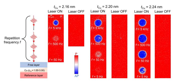
FIG. 4. The P-to-AP switching obtained by constant excitation with various frequency f. MOKE images obtained during constant excitation (Laser ON) and after the excitation (Laser OFF). The laser fluence used for the experiment is around 7.8 mJ/cm<sup>2</sup>.
