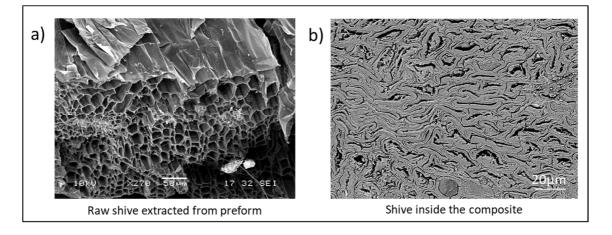
Figure 4: SEM observation of a shive a) before the composite manufacturing step with open cells, b) after composite manufacturing, showing collapsed cells.
