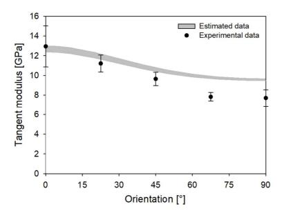
Figure 7: Evolution of the tangent modulus with loading orientation for non-woven flax/PLA with 50wt% of fibres tested in tension.
