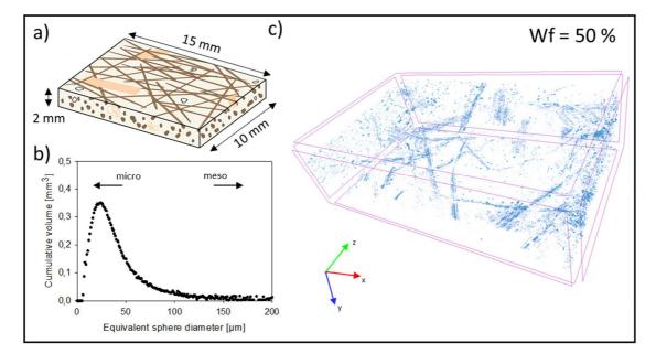
Figure 3: Porosity analysis by micro-CT a) schema of the analysed sample, b) analysis of porosity size, c) the micro-CT 3D view of porosity.
