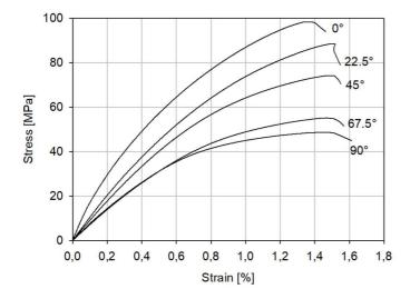
Figure 6: Tensile behaviour of non-woven flax/PLA with 50 wt% of fibres at several loading angles. The 0° refer to the machine direction and the 90° to the cross direction.
