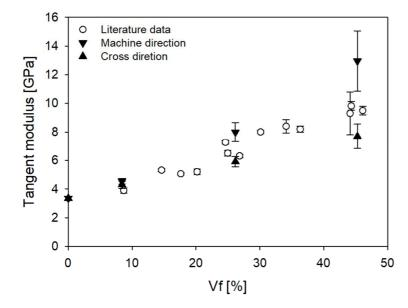
Figure 8: Evolution of tangent modulus with fibre volume fraction, with measurements in the orthogonal machine and cross directions presenting anisotropy. A comparison with literature data is also presented.
