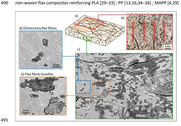
Figure 2: SEM observation of the flax/PLA non-woven investigated, a) a schematic representation of the analysed sample, b) upper observation, showing preferential fibre orientation (red arrows), c) transverse observation, cracks might be due to water polishing, d) zoom on elementary flax fibres, e) zoom on flax bundles.
