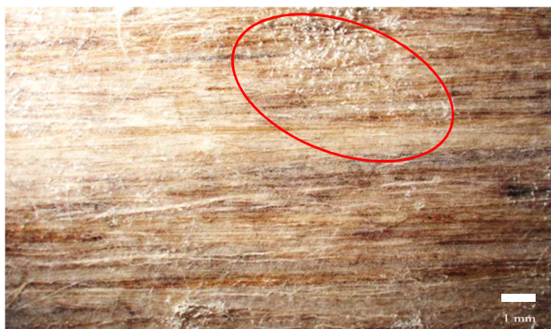
308 Fig. 4 - Pictures of the surface of flax/PP+MAPP asymmetric samples after conditioning 15 days at 99 %RH. 309 The red circle highlights the appearance of mold. 310
